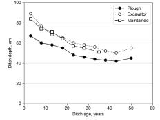
Figure 1. Average depth of original ditches made by plough or excavator, and maintained ditches made by excavator as a function of ditch age
