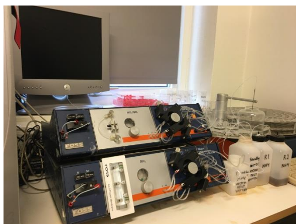
Figure 6. Flow injection analyser (FIA) used for determining ammonium-N in solution (Photo: Åsa Myrbeck).
