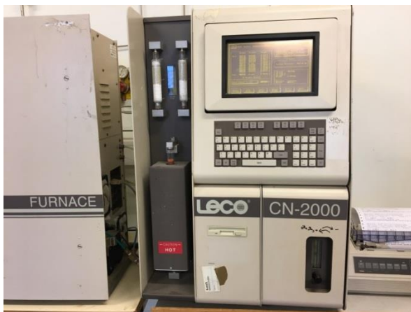
Figure 8. Unit used for measuring total carbon and nitrogen content of dry samples with Dumas method (Photo: Åsa Myrbeck).
