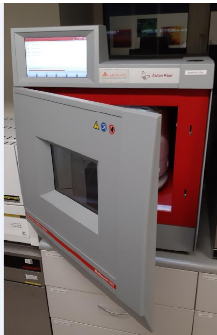
Figure 7. Microwave oven to digest samples with acid (Photo: Lauris Leitans), and samples that have been extracted with nitric acid (Photo: Åsa Myrbeck).
