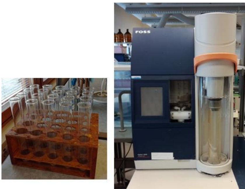
Figure 4. Kjeldahl system. Left there are macro-Kjeldahl tubes used in digestion and right there is a distillation and titration unit. (Photo: Tapio Salo)
