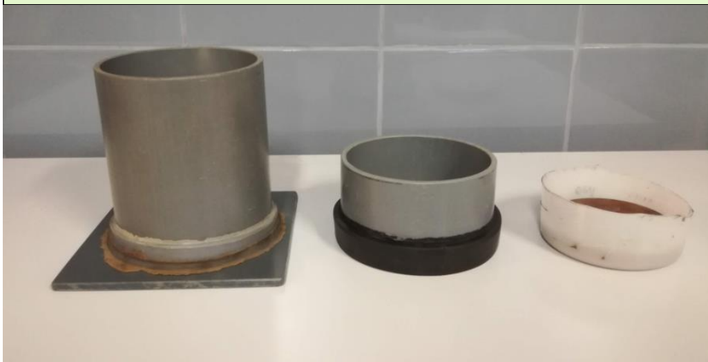
Figure 10. Test cylinder of one litre, removable collar and weight used in volume weight measurements. (Photo Tapio Salo).
