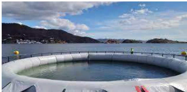
Figure 58. The picture shows the closed sea pen tested by the company Nekkar AS in Flekkefjord in the period 2021-2022.
